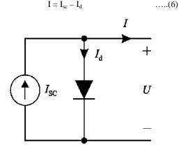
Fig. 2. Electrical circuit diagram representing the onediode model of an ideal PV cell.
