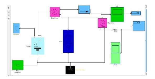
Fig. 4. Diagram of the MATLAB-Simulink based PV module model.
