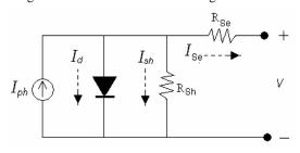
Fig. 3. Electrical Model of PV Cell.
